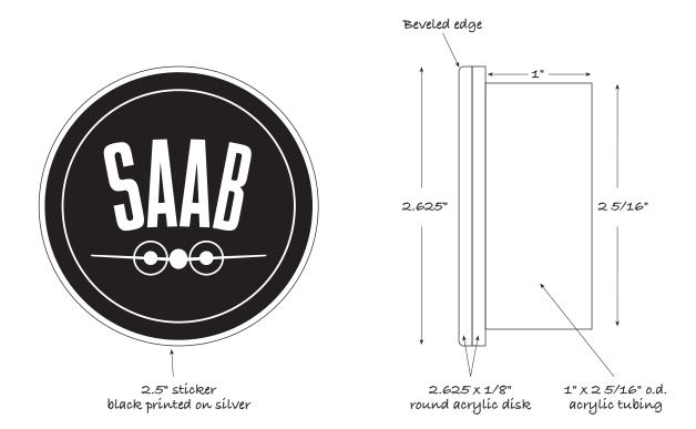
The 2.625" x 1/8" round acrylic disks are glued together with the SAAB sticker between them and then this assembly is glued to the 1" x 2 5/16" o.d. acrylic tube. The tube slides into the wheel opening and is epoxied in place.
